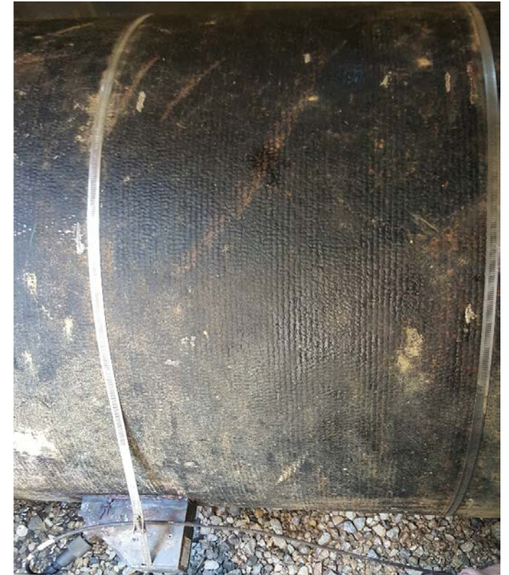
Transit Time ultrasonic meter with strap-on transducers on the pipe exterior
