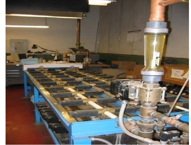
Large test benches that can test many meters at one time
