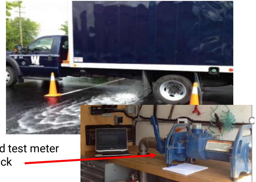
Meter testing via truck mounted apparatus (Courtesy of Louisville Water Company)
